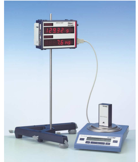
The Cobra3 DISPLAY UNIT can even be used as a demonstrative remote display for scales (Sartorius /Scaltec).
