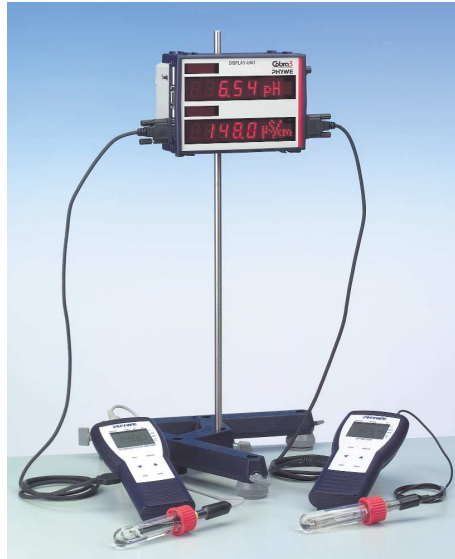
If two hand-held measuring devices are connected, 2 measured values can be simultaneously displayed with their units.
